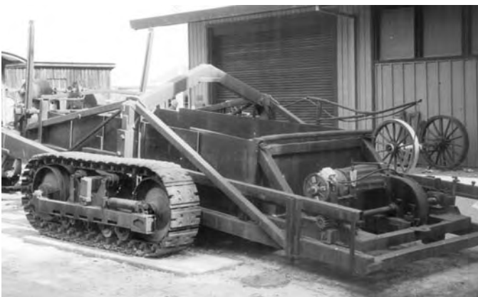
One of Richard LeTourneau's Telescopic Scrapers. This one is at the San Joaquin Historical Society Museum at Micki Park near Lodi, California. It is virtually identical to one of the three such scrapers that were towed over the PG&E Road in 1926. Author
